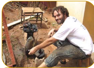
Using Grandpa Huntoon's hand-crank bellows and crucible to heat up the solder for the battery connections over a charcoal fire
