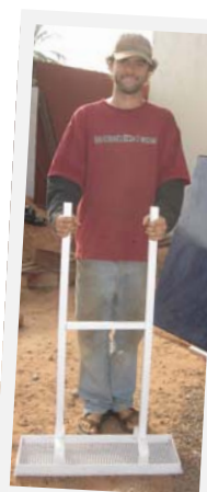
Jason's new jitterbug-welded, sanded, painted, and ready to go
