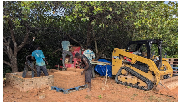
The block maker is now powered by electricity instead of diesel and is more reliable and much quieter!
