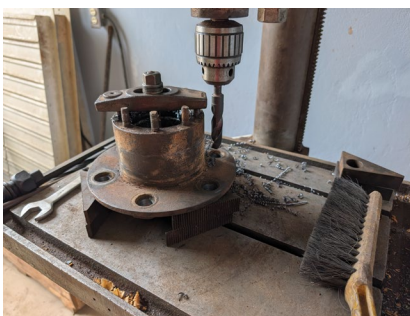
Drilling out the holes for replacement wheel studs in a truck's hub.
