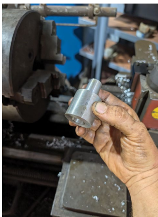
Sometimes the projects are to keep our own vehicles going! In this case we couldn't find a replacement battery for the skid steer with a flat top like the original, so I had to machine a battery post extension so the connector could clear the raised top of the new battery!
