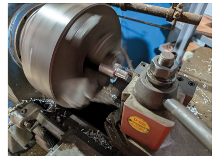
Sometimes the projects are to keep our own vehicles going! In this case we couldn't find a replacement battery for the skid steer with a flat top like the original, so I had to machine a battery post extension so the connector could clear the raised top of the new battery!
