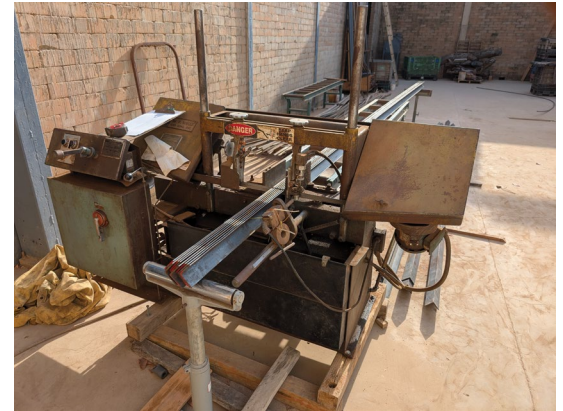
This Wells bandsaw made in Kalamazoo, MI in 1983 is the best horizontal bandsaw my workshop has had. It chews through stacks of stock making clean, straight cuts. Sure beats a hacksaw and a sore arm!
